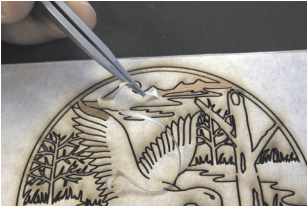
7. Carefully remove the **application tape to expose the areas that you want to be gold gilded.
