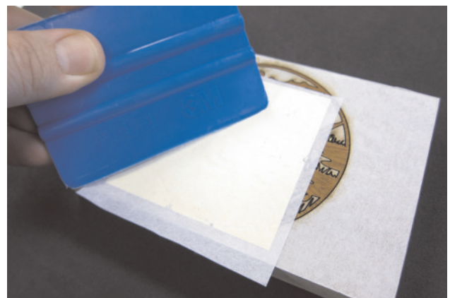
12. Press the gold leaf onto the part, a squeegee may be helpful to get a firm adhesion.
