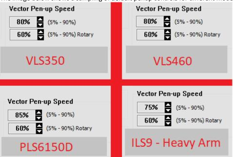
If the UCP is newly installed on a computer that has never had a ULS driver on it previously, then the default pen up speeds will be loaded as soon as the engraver is connected to the computer and powered up.
