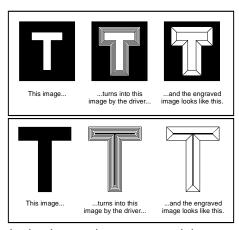
To obtain a "chiseled" or "sunken" engraving, create a "positive" graphic so that the background is white and the text or objects are black. This way, the text or graphic engraves and the background remains untouched, producing a "chiseled" effect.
