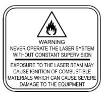
Acrylic is extremely flammable. Do not leave the laser system unattended when cutting or engraving.
