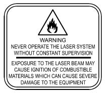
Acrylic is extremely flammable. Do not leave the laser system unattended when cutting or engraving.
