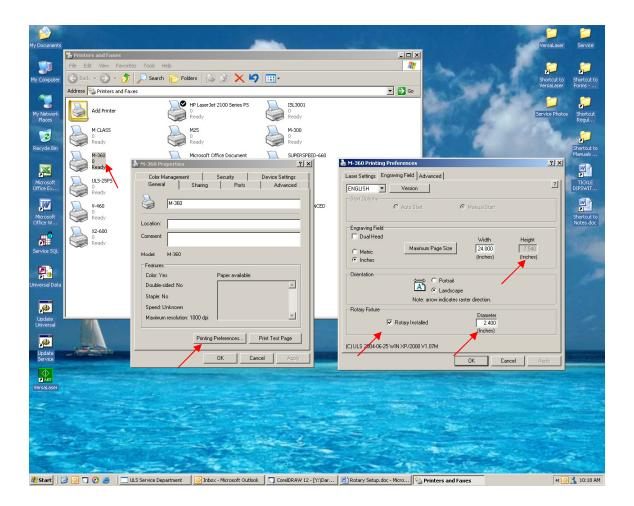
11) Input diameter of part to be marked. Example 2.4"
