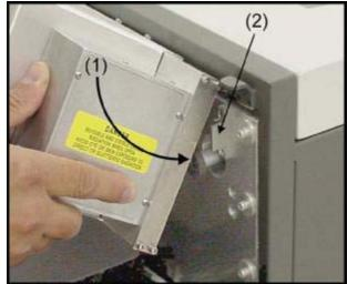
4) Pick up the laser cartridge by the sides and tilt it downward on a 30-degree angle. Mount the cartridge onto the mounting blocks by placing the upper "V" groove on top of the mounting blocks. Slide the cartridge to the right until the **OUTER EDGE** of the alignment plate contacts the **INSIDE EDGE** of the large plate of the alignment fork.
