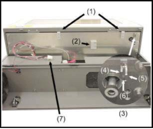
2) Visually locate the two mounting blocks (1), the laser latch (2), alignment fork (3), and power connector (7). Notice that the alignment fork has two plates, one small (4) and one large (5). Locate the gap between the two plates (6).
