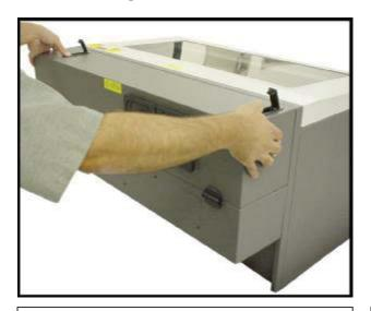
1) Make sure that your power cord **IS NOT** plugged in at this time. Press on the backside of the two hinges to release the latch. Gently fold back the rear cover.
