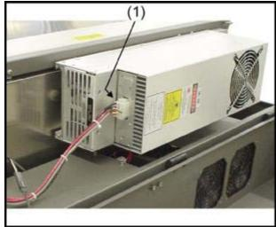
5) Slowly rotate the laser cartridge making sure that the alignment plate is centered in the gap of the alignment fork between the small and large plates. As you slowly release the weight of the laser, you should feel it lock (clunk sound) itself into place, parallel to the mounting surface. Make sure that you do not pinch any wires or hoses. Verify that the, alignment plate is centered within the alignment fork.
