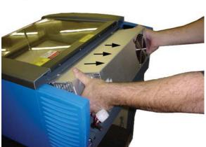
**4.** Rotate the laser, a few degrees, from the bottom and lift it up and off the mounts. Store the laser in a safe place.
