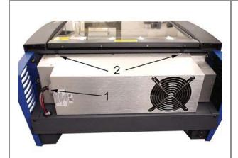
3. Unplug the white electrical connector (1), from the Laser, by squeezing its locking tabs and pulling it to the left. Remove the 2 screws (2) that attach the Laser to the frame.
