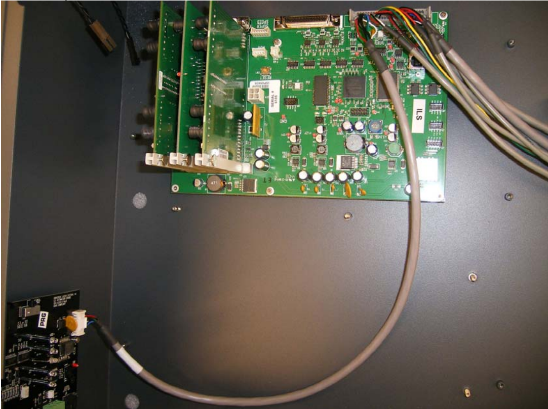
With Standard Air Assist: Connect Automation Kit J1 to CPU J1 “Accessory” cable
