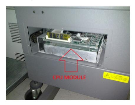
Step 3 – Look for the **Fail Safe** Button as shown in the picture. Disregard the Reset button in the picture shown below; most new CPUs do not have a Reset button but a **Fail Safe** button only. Plug the main power cord back into the engraver.
