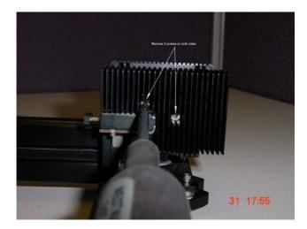
Remove the 4 screws shown in Figure 1. Remove the 2 screws shown in Figure 2, you will find 2 additional screws on the opposite side.
