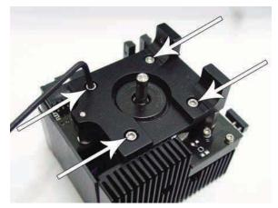
**8.** Loosen the 4 mounting bracket screws. Once you remove the screws **do not** pull on the bracket as it is still attached with a wire connector.
