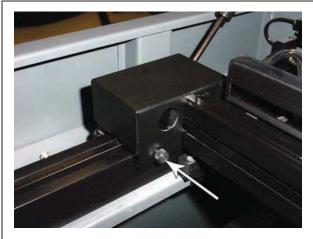
1. Remove #2 mirror cover by removing the thumbscrew and sliding the cover to the right and up.
