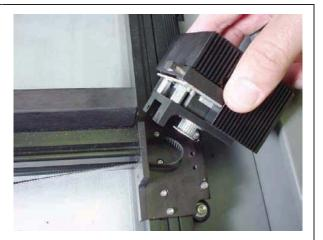
**4.** Remove the other mounting screw (5) is on the front side of the motor housing with a 3/32 Allen wrench. Lift the motor housing off of the arm and put it on a table in a safe place. Be careful not to drop the Motor Module or touch the Y-axis home sensor.
