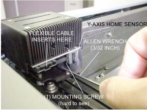
2. The other mounting screw is on the front side of the motor housing. Also remove this screw with a 3/32 Allen wrench. Lift the motor housing off of the arm and put it on a table in a safe place. Be careful not to drop it or touch the Y-axis home sensor.
