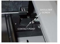
• If there is a gap between the shoulder screw and the contact point on either the left or right side of the arm, you will need to square the arm by making an adjustment.
