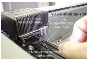
3. Using a 3/32 allen wrench remove the 4 socket screws, 2 on each side of X axis arm. Store the screws in a safe place.
