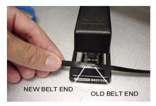
Using belt tool, adjust tension to specification by tightening or loosening Y axis idler located at the back of both Y axis rails. Please refer to the attached belt tension document. Adjust both tension screws equally. Failing to do so will result in Y axis belt tracking incorrectly.
