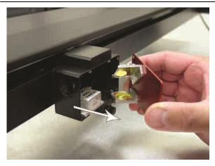
2. Remove the optics from the Focus Lens Carriage by unscrewing the 2 thumb screws and pull the face plate out towards you. Place the optics in a safe, clean place.
