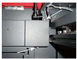
11. Next, undue the two large screws that cover the X-Axis Motor with a flat head screw driver. The screws will not come apart from the cover. Set the cover aside.
