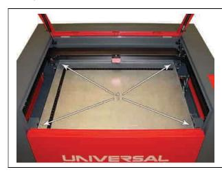
Locate and remove the eight screwsfound on the top surface of each corner of the table.
