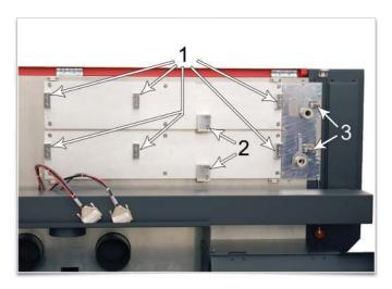
**3.** Locate the "V" groove along the upper (3) and lower (2) part of the laser cartridge base plate and the alignment plate (1) at the end of the base plate.
