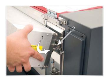
**6.** Slowly rotate the laser cartridge, making sure that the alignment plate is centered in the gap in the alignment fork. As you slowly release the weight of the laser, you should feel it lock itself smoothly into place. Never force the laser into position. If the laser does not install smoothly, check for obstructions such as pinched wires or hoses or a binding laser latch. Once installed, verify that the alignment plate is centered within the alignment fork.
