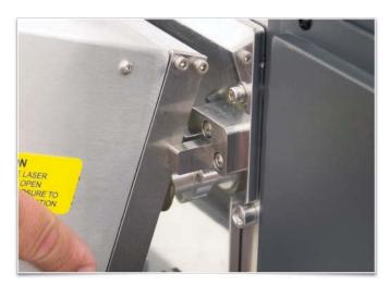
7. Plug in each power connector (1) to the corresponding laser cartridge. The power connectors are labeled Top (2) or Bottom (3). Single laser cartridge users will use the top laser connector only.
