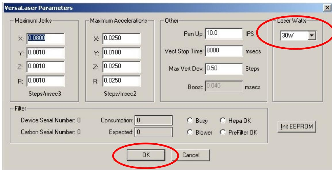
3. From the dropdown list “Laser Watts”, select the new wattage to be programmed.
