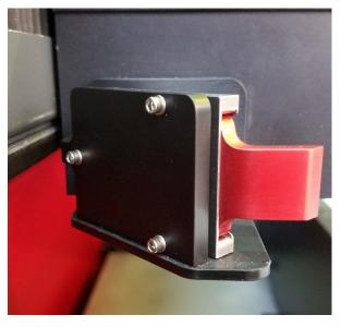
8. Once centered, remove alignment tool. Reinstall the #1 XLS MWH Turning Mirror Assembly.
