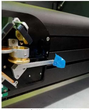
7. Under System Configuration "Alignment", select center location of table. Activate laser 1 using only enough power to discolor the tape. Usually 5% power .3 second. If centered or near center, you're aligned well enough. If not, on the left side of arm adjust the 3 5/64<sup>th</sup> socket head cap screws located on the back of the #2 mirror until centered. Use red diode for alignment reference.
