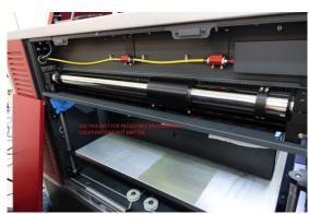
6. Use the ¼" bolt to increase the tension of the Y axis belt. The belt tension should be 45-50 hz. If there is no gap left the belt tension cannot be increased and a tooth will need to be removed from the belt.
