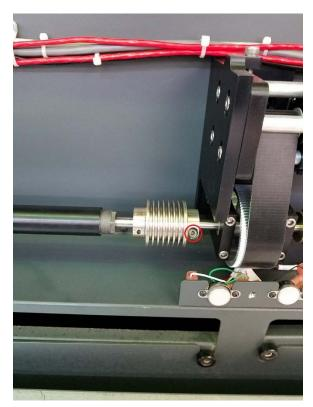
5. Push arm toward the rear of system until both right and left sides hit the hard stops. Left side shown.
