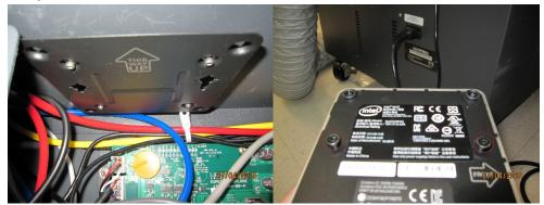
6. Install the USB 2 Cable Straight A to down angle B. You may need to remove the gray front panel. Mounting screws are circled
