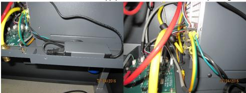
4. Navigate the NUC side of the Power Supply to the mounting side of the system.
