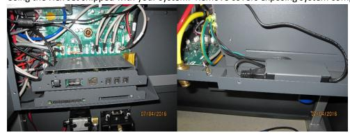
3. Mount and wire the NUC Power Supply as shown below. Green always being Ground.
