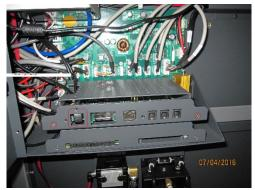
7. Next install Ethernet Panel mount 1' using hardware supplied.
