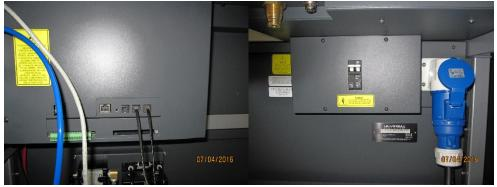
2. Using the Hex set shipped with your system. Remove covers exposing system components.
