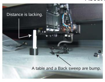
1. When a "back sweep" is installed, "2 inch lens" can not be in focus. Because, a table and a Back sweep will bump. It will be satisfactory if it is a lens more than "3 inch." Or probably, the length of stay of a "back sweep" must be changed.
