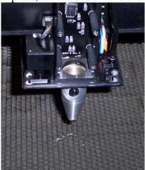
Step 3: Connect air tubing located on the right side of the cone to the barbed fitting attached to the focus carriage plate.
