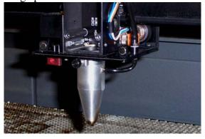
Step 4: Reinstall your cover removed in Step 1. Remember to remove Air Assist Cone when not using air assist. Failing to do so will cause damage to focus lens.
