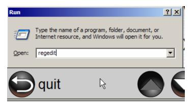
When **regedit** launches, navigate to the Registry key called HKEY\_LOCAL\_MACHINE\SOFTWARE\ULS, as show below.
