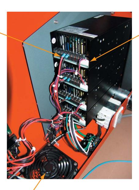
When 4 plugs were unpluged and laser was irradiated, this cooling fan became slow-down.
