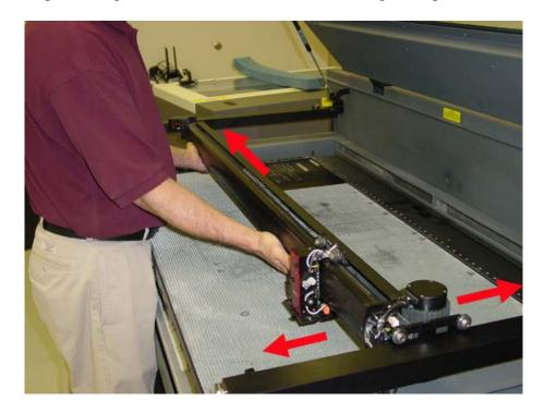
8) Installation of the new arm is in reverse of removal. Airline installation will require the use of a pair of forceps that have had the jaws wrapped with electrical tape. This will allow the hose to be gripped while installation, but not rupture the hose.
