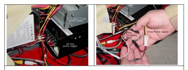
8) Connect the power connections. The ring terminals install in the same location as the previous air assist power connection on the 48 volt power supply. The 12 volt connector (Green and yellow two pin wire connections) splices into the 12 volt harness as indicated.
