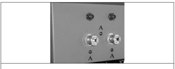
5) Remove the screws holding the air assist controls in place.
