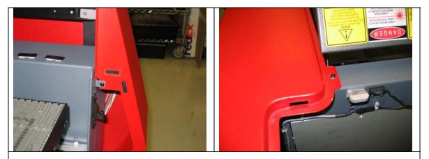
2) Remove the cover screws the hold the right side panel. You will need to open the laser door and the front door to access the screws.
