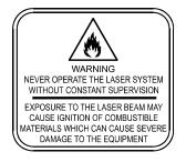
LASER ENGRAVING OR CUTTING PLASTIC CAN IGNITE THE MATERIAL. Never leave the laser system running unattended for any reason.
