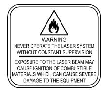
Acrylic is extremely flammable. Do not leave the laser system unattended when cutting or engraving.
