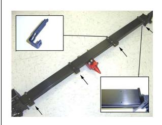
5. Attach the L-brackets to the back of the X rail with the silver Phillips screws included in the upgrade kit (two for each bracket).
