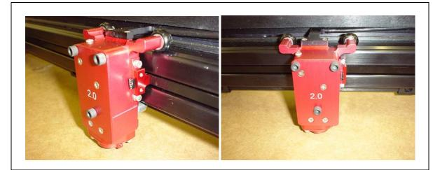
1. (Remove Optics First) Remove the focus carriage from the X-axis arm on your machine by first detaching the belt clip from the right side of the carriage by removing the two screws on the ends of the clip. Next, hold the carriage on the bottom with two fingers and your thumb on top, gently lift up and pull the carriage off the rail.
