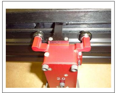
14. Attach the focus carriage to the air track slider manifold using Allen screws
