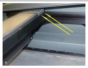
**1Q** Locate and carefully remove the two screws securing the cover on the <u>left-hand</u> side of the X-axis arm. Remove this cover.
