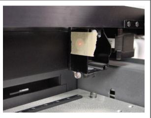
**14** With the cover removed, locate the three adjusting screws on the #2 Mrror mount on the left-hand side of the X-axis arm. Turn these screws to center the red dot diode.
