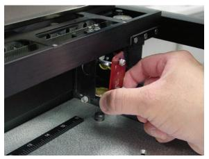
**2** Remove the optics from the Focus Lens Carriage and place in a safe, clean place.
