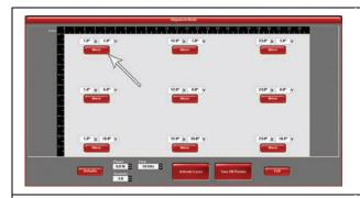
**13** Click on the upper left hand Move button. The VLS's focus carriage will move to the indicated X, Y position.
